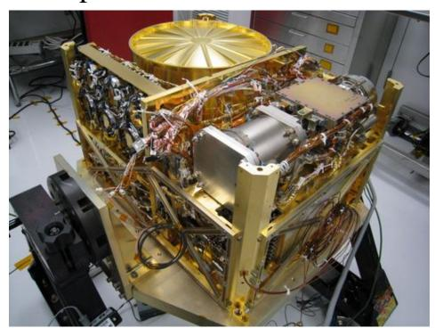
The Sample Analysis at Mars (SAM) instrument, at NASAâ $\in$ <sup>TM</sup>s Goddard Space Flight Center, Greenbelt, Md., will analyze samples of material collected by the roverâ $\in$ <sup>TM</sup>s arm. Credit: NASA/JPL
