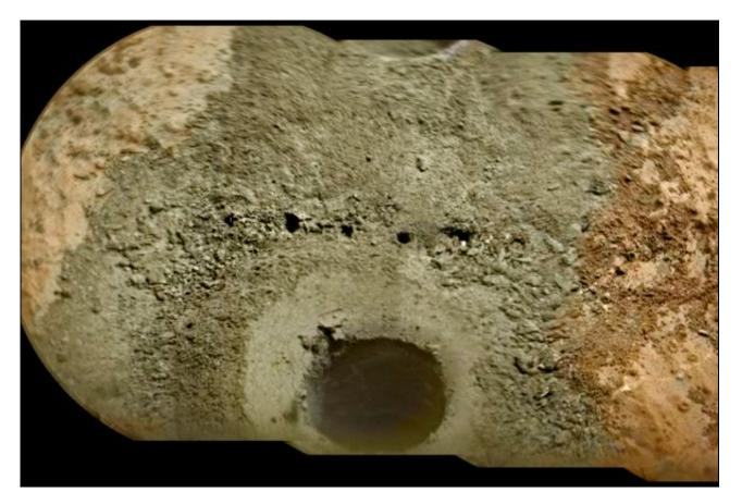
The Curiosity rover used a laser to sample freshly drilled rock dust on Mars.
