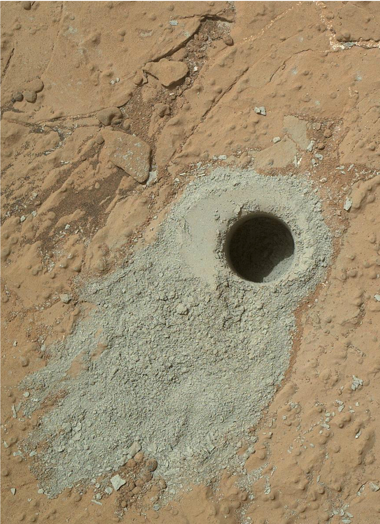
Curiosity detected organic molecules in a powder sample collected in May 2013 from a rock named Cumberland — the first definitive detection of organic chemicals on the martian surface. Credit: NASA/JPL-Caltech/MSSS
