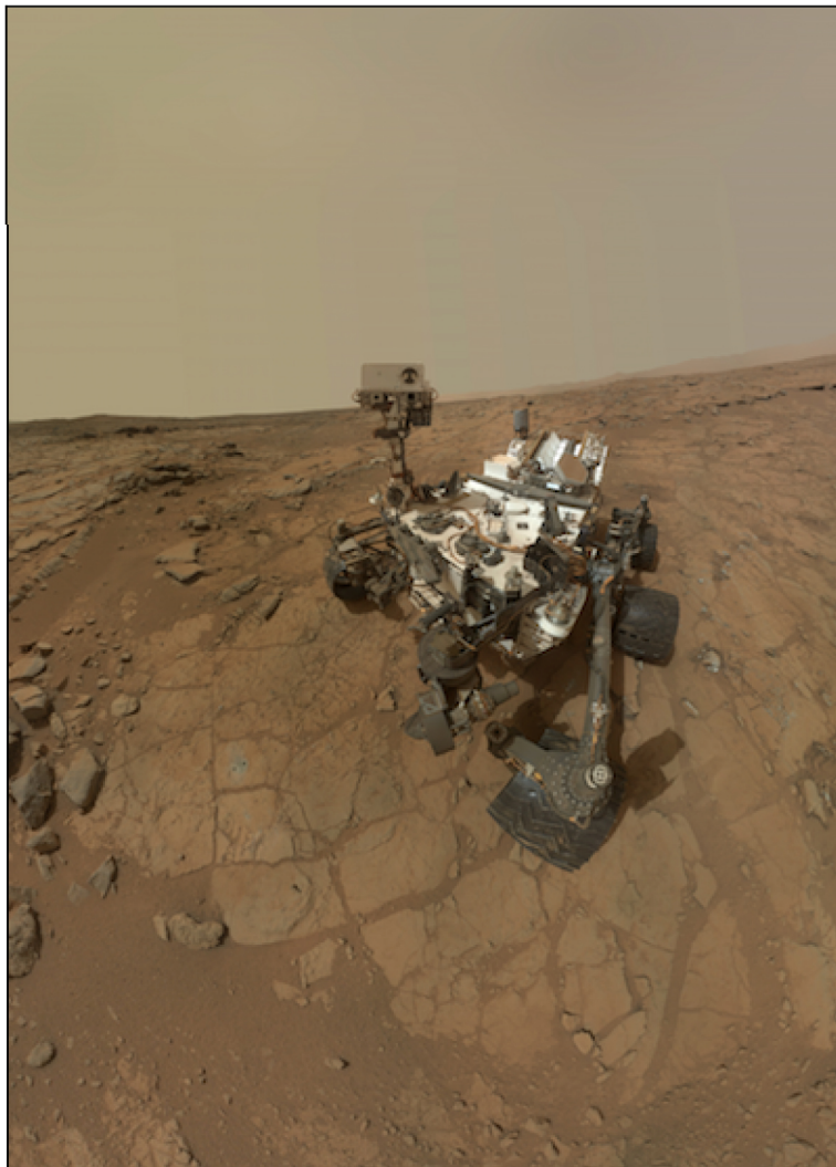
The rover's Mars Hand Lens Imager took dozens of exposures to be compiled into this mosaic self-portrait while Curiosity was stationed at a work site named "John Klein" earlier this year. Credit: NASA/JPL-Caltech/MSSS
